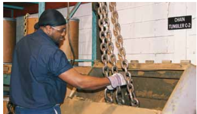
Cleaning the chain for inspection.
