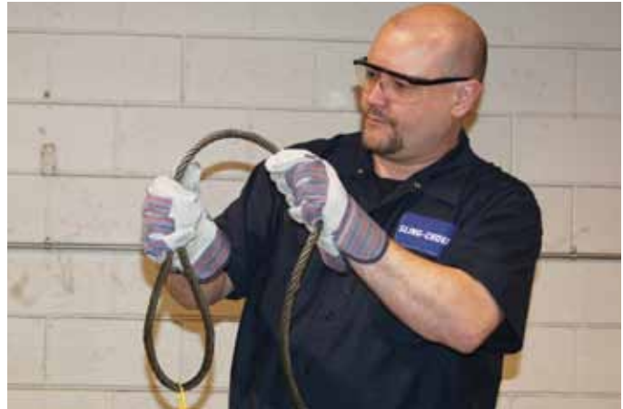
Visual inspection of a wire rope sling
