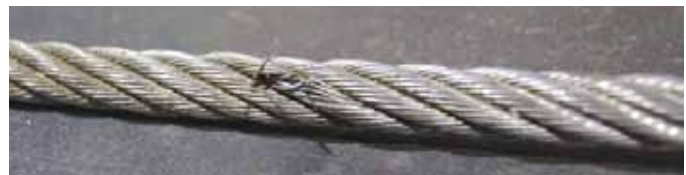
Example of broken wires
