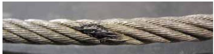
Example of heat damage
